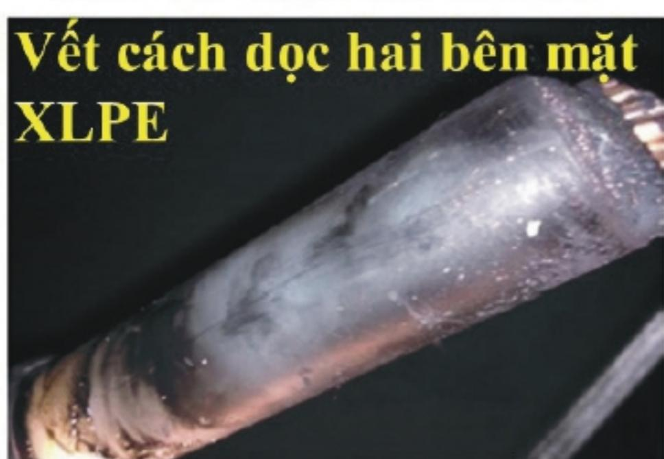
Picture 5 The 2nd longitudinal knife cut on the XLPE
